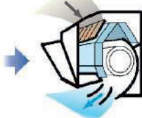
Cooling Operation To make condensing water.
